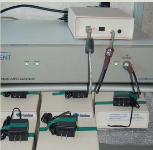
GNSS RF recorders with OCO under test with single-channel GPS simulator
