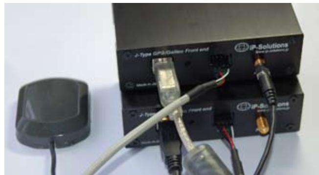
Two RPSes: The bottom unit functions in playback mode while the top one is operates as a front end for a PC-based software receiver
