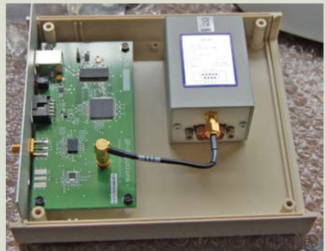
GNSS RF recorders with OCO under test with single-channel GPS simulator
